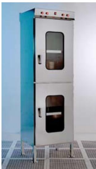
Ultraclean N2 purging cabinet - Dessicator, is fully automated allowing full control of N2 input according to requirements. This is the ideal solution for low humidity storage. This unit is specifically designed for four 300mm FOUP pods. This cabinet is typically used to store pre purged FOUP pods for long periods of storage. Fabrication material : 304 sst, electropolished. High purity materials.
